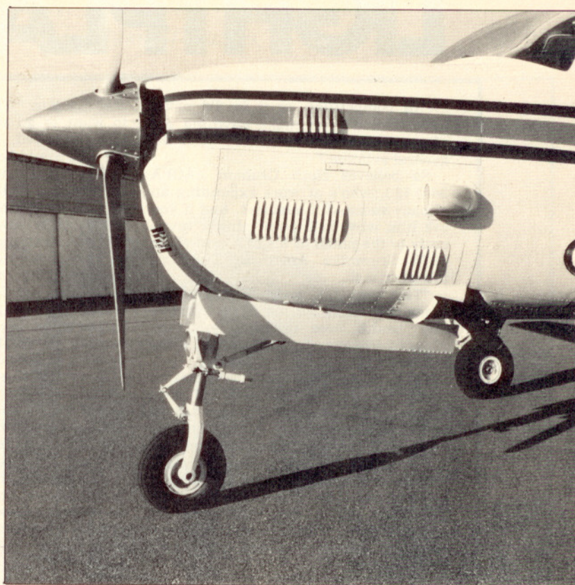
The A36TC bristles with gills, louvers, lips and air intakes to get away from cowl flap drag
